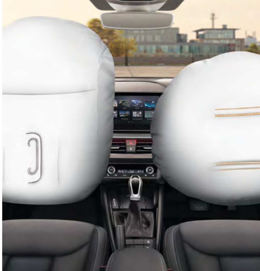
Front airbags While the driver airbag is enclosed in the steering wheel, the passenger airbag is located in the dashboard.
