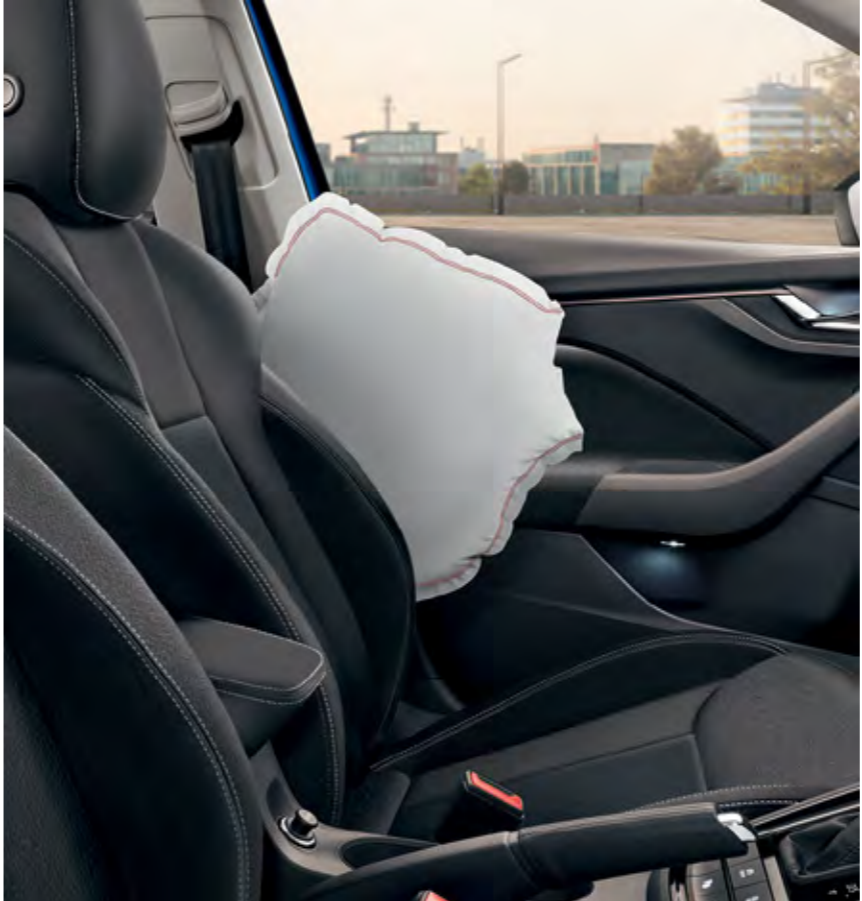
Front side airbags These two airbags protect the pelvis and chest of the driver and front passenger in the event of side collision.
